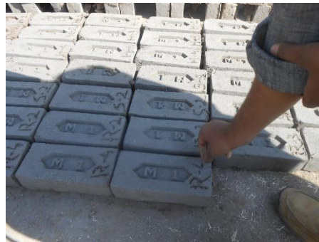
Fig 3.3.1. Naming of Each Brick
