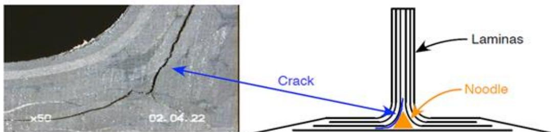
Fig. 1 Crack Propagation in Laminated Composites
