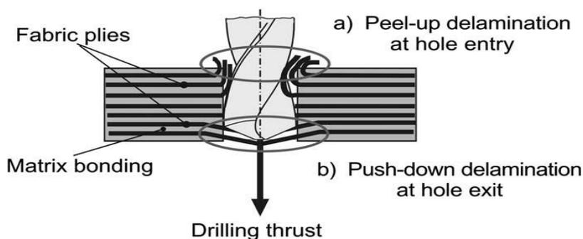
Fig. 4 Classification of delamination.<sup>[11]</sup>
