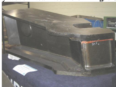
Fig. 6 – Metal: 335kg Carbon: 285kg Weight Saving – 15% Fig. 7 Material Distribution in standard vehicle
