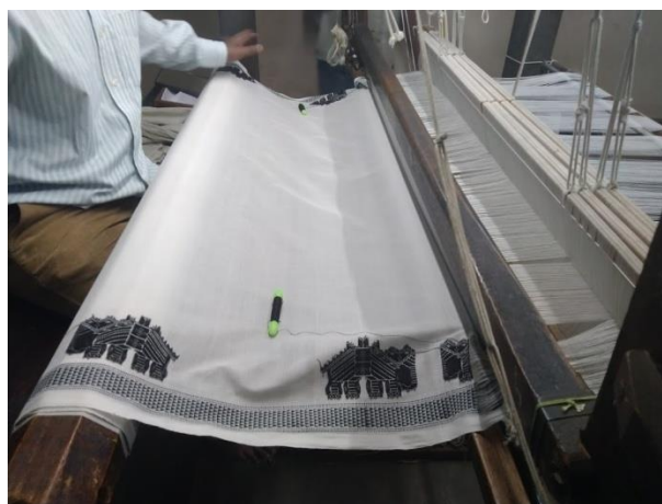
Fig. 6. Saree in a handloom - visibility of the wrong side of the saree-elephant motif and border
