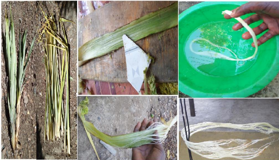
Figure 2: Pineapple leaf fiber extraction by scrapping method
