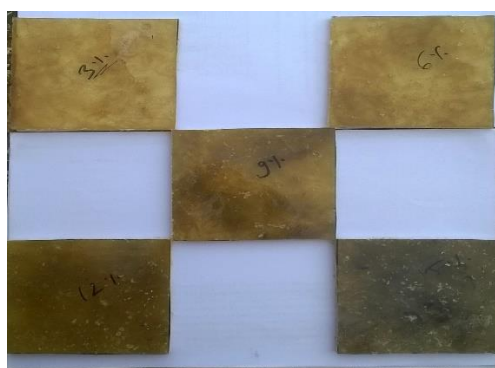
Fig- Composite sheets with different weight fraction of mulberry re-reeling silk waste.
