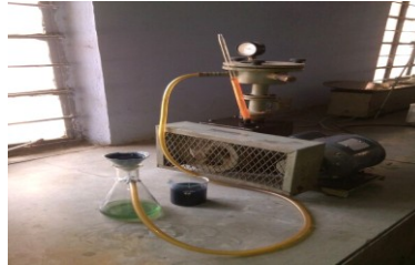
FIG. 2.2 - ASSEMBLY WITH SUCTION PUMP AND VACUUM FLASK EMPLOYED FOR FILTRATION AND RECOVERY OF INDIGO
