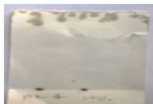
FIG.3.3 - COMPARISON BETWEEN INDIGO STANDARD AND PH – 14 & PH – 4 ON T L C PAPER
