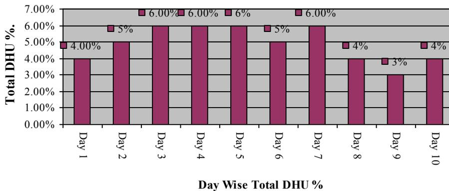
Graphically shows day wise garment rejection % after corrective action, which reduces the defect rate in top five defects like Skip Stitches, Puckering, Measurement, up down, other defects so it help to reduced DHU % .
