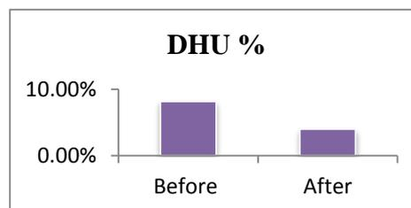
We change the sewing machine setting like reset tensioner, synchronisation in loopformation during stitching , awareness in operators about physical properties of fabric which help to reduce DHU%. As per this graph overall DHU of before trail are 8% and after carried out experimental work it can be reduce by 4%. Overall DHU of after trail are 4%.
