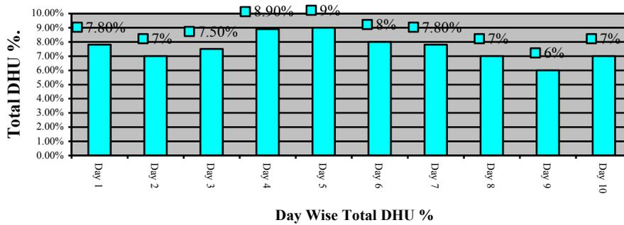
Graphically shows day wise garment rejection % due to various reasons like skip stitches, up down, stains, puckering and measurement and other defects because of these defects total DHU is 8% which is higher than normal range.
