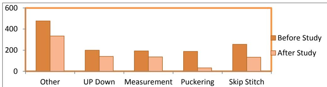
This graph shows defects like other, up down, measurement problem, puckering and skip stitches were more before trail due to problems in sewing machine setting like tensioner, time synchronisation during stitch formation, awareness in operators about physical properties of fabric.
