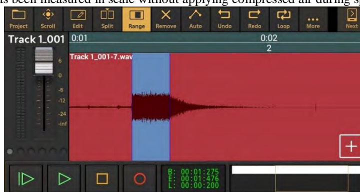
Figure 1. Valve opening time calculation by sound wave method
